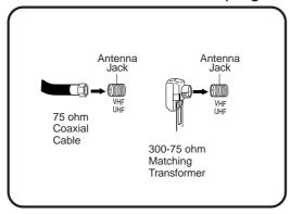
Connect the 75 ohm cable from the combination VHF/UHF antenna to the Antenna Jack.
